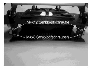
Ill. 10 M4x12 countersunk screw M4x8 countersunk screw
