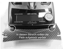
Ill. 5 Pads should be applied (glued) in this area
